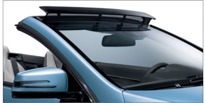
The air deflector of the AIRCAP system directs the airflow over the interior in an arc. It extends at the touch of a button and retracts automatically
