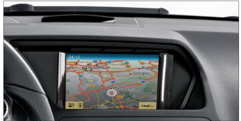
Entertainment at your fingertips: the multimedia system COMAND APS helps the car to navigate and is equipped with a radio, CD/DVD player and Aux-in socket
