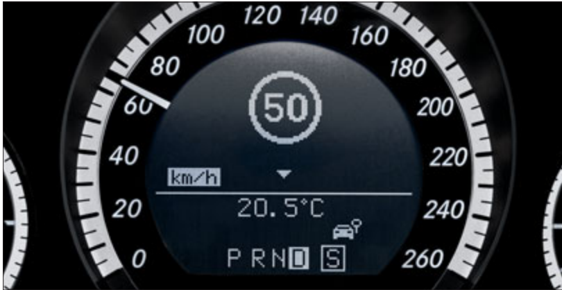
Speed Limit Assist (optional) identifies the signposted speed limit and displays it in the instrument cluster
