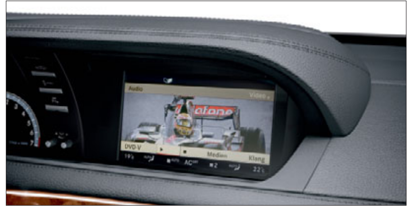
SPLITVIEW offers the driver and front passenger two different programmes at the same time on a single screen
