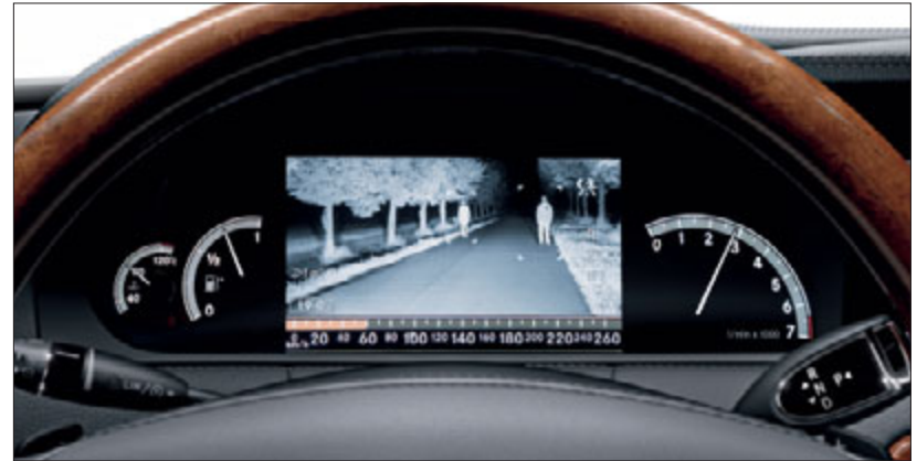
Thanks to infrared technology, Night View Assist Plus is able to detect pedestrians who are up to 90 metres away
